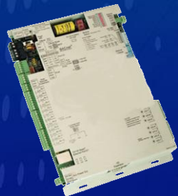
Existing HVAC System Controller
