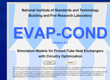
Simulate heat exchanger performance with PIV data and employ evolutionary algorithms to modify refrigerant circuitry for optimal capacity
